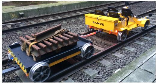
Gauge: Standard 1435mm (other gauges available) Frame: Welded rectangular tube . aluminium.
