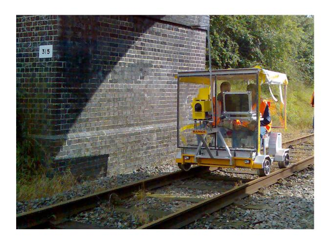
For the accurate mapping of track structures and tunnel clearance.
