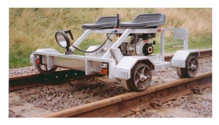
Gauge: Standard 1435mm (other gauges available) Frame: Welded rectangular tube - aluminium.
