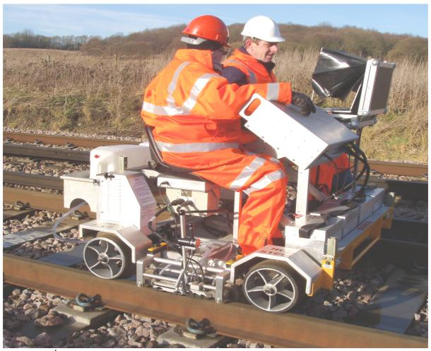
\*photograph shows UTV with sliding probes (wheel probes available as per photograph overleaf)
