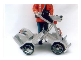
One ultrasonic screen is used for each rail. Defects are indicated on the screens concurrently with audible warnings and a flashing light.
