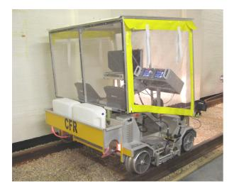
Two floodlights and one spotlight are standard equipment for night working. Automatic red and white direction marker lights are also standard.
