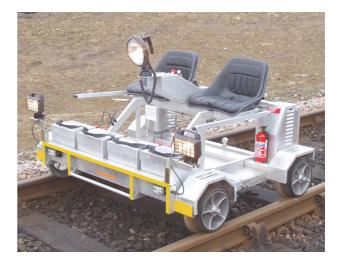
The UTV is light enough for 2 operators to handle easily. The components are small enough to be transported in a small van and for getting to the track down stairways, etc. The vehicle and ultrasonics can be assembled in five minutes
