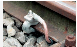
Electrical rail contact with reusable and vibration-proof M10 nut and cable lug for return currents, mast grounding, signal circuits etc. Advantages: Fast and easy cable fitting, larger contact area.
