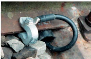
Electrical rail contact tapped for vibration-resistant M12 screw fixing and cable lug, for return currents, mast grounding, signal circuits etc.
